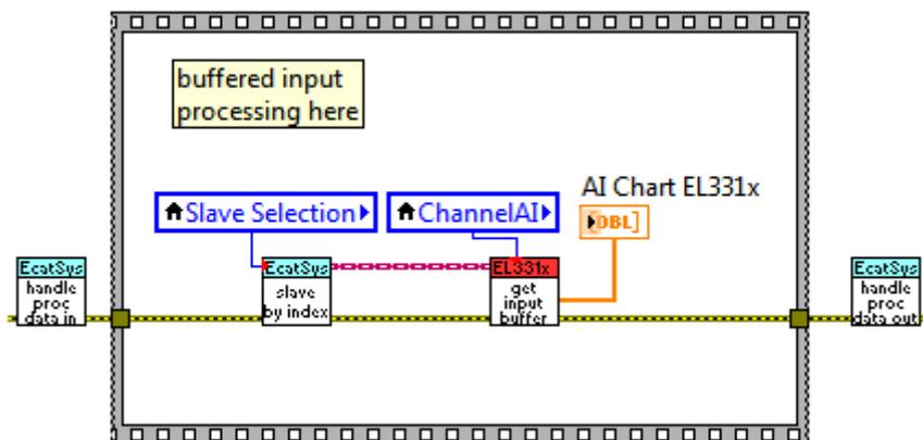
The function handleProcessDataOut writes the output data of the slave objects to the output process data and sends it to the bus.
