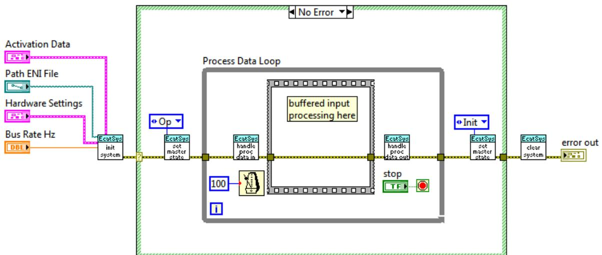
The basic structure for running the EtherCAT bus is:
